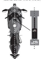
3. Keep both bike wheels on the ground. Adjust the mount plate till it is parallel to the ground. Adhere the plate to the gas tank.
