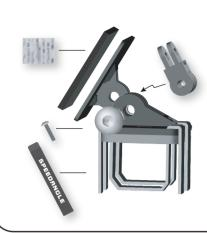
2. Adhere the two Dual Lock strips to the back of APEX.
